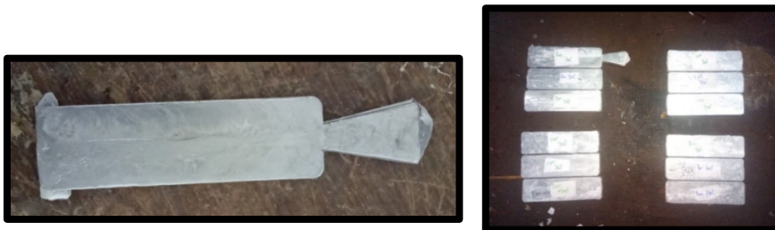
Figure 2. Casting result produced by stir casting method with metal mold
